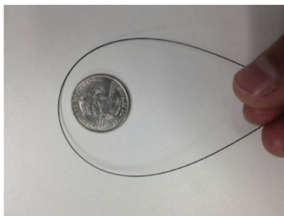
Fig. 10. Typical CMS fiber showing remarkable flexibility. (A colour version of this figure can be viewed online.)
