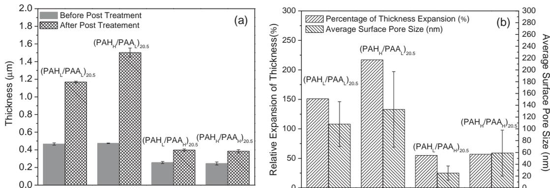
**Figure 2.** a) Thickness of thin films before and after the post-treatment and b) the relative expansion of thickness and average surface pore size for (PAH<sub>L</sub>/PAA<sub>L</sub>)<sub>20.5</sub>, (PAH<sub>H</sub>/PAA<sub>L</sub>)<sub>20.5</sub>, (PAH<sub>L</sub>/PAA<sub>H</sub>)<sub>20.5</sub>, and (PAH<sub>H</sub>/PAA<sub>H</sub>)<sub>20.5</sub>, respectively. All the films were fabricated using deposition time of 10 s.
