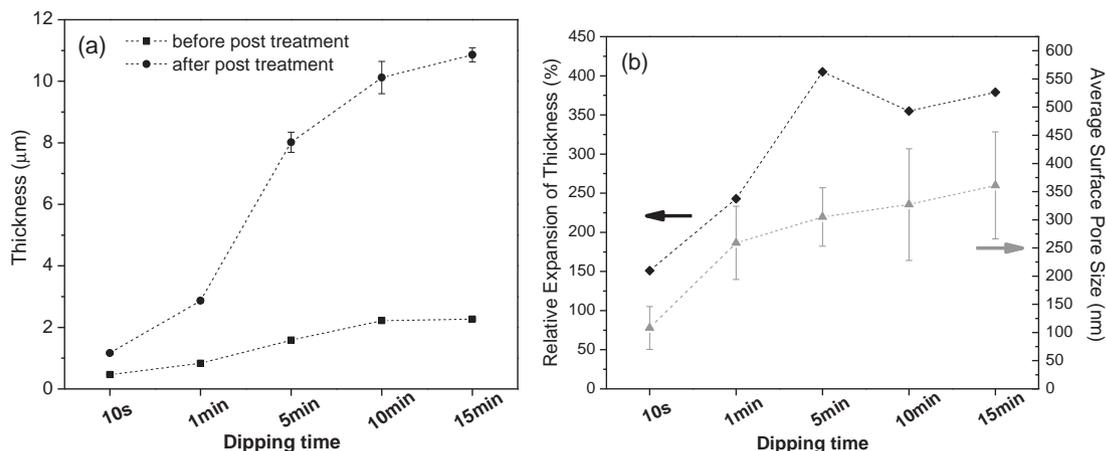
**Figure 1.** The effect of deposition time on a) the thickness of PAH<sub>L</sub>/PAA<sub>L</sub> thin films before and after the post-treatment and b) the relative expansion of thickness and average surface pore size.
