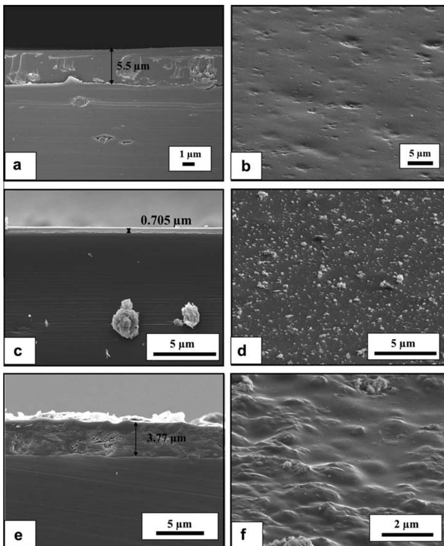
**Fig. 2.** SEM micrographs of 20 bilayer GNP embedded PEM assembly. a, c, e show sectional view of hydrogen bonded, electrostatic, and composite (10H + 10E) multilayers, respectively. Thickness of the coating is 5.5  $\mu\text{m}$ , 0.705  $\mu\text{m}$ , and 3.77  $\mu\text{m}$ , respectively. b, d, f show surface morphology of hydrogen bonded, electrostatic, and composite films, respectively.
