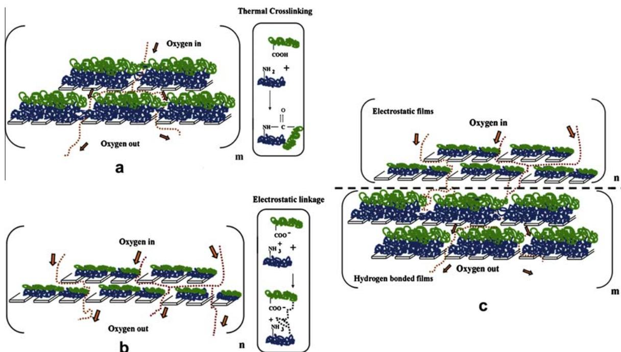
**Fig. 1.** Supramolecular assembly of graphene embedded polyelectrolyte multilayers. (a) Multilayers assembled using hydrogen bonded assembly.  $m$  denotes number of bilayers deposited. (b) Multilayers deposited using electrostatic interactions.  $n$  denotes the number of electrostatic bilayers deposited. (c) Composite film consisting of “ $m$ ” number of hydrogen bonded bilayers followed by “ $n$ ” number of electrostatic bilayers.
