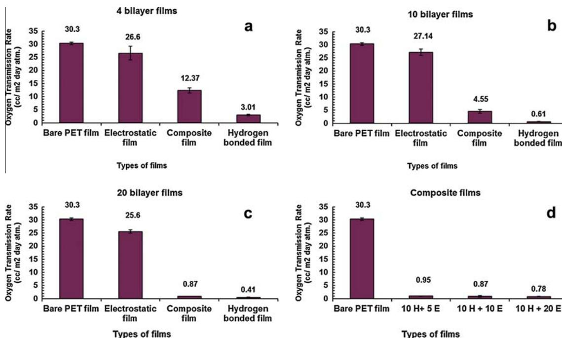
Fig. 3. Oxygen transmission rate (OTR) for different types of configurations. (a) Four bilayer system. The composite film consists of 2 hydrogen bonded and 2 electrostatic bilayers. (b) Ten bilayer system. Composite film consists of 5 hydrogen bonded and 5 electrostatic bilayers. (c) Twenty bilayer system. Composite film consists of 10 hydrogen bonded and 10 electrostatic bilayers. (d) Composite films consisting of 10 hydrogen bonded (H) followed by varying number of electrostatic (E) bilayers.
